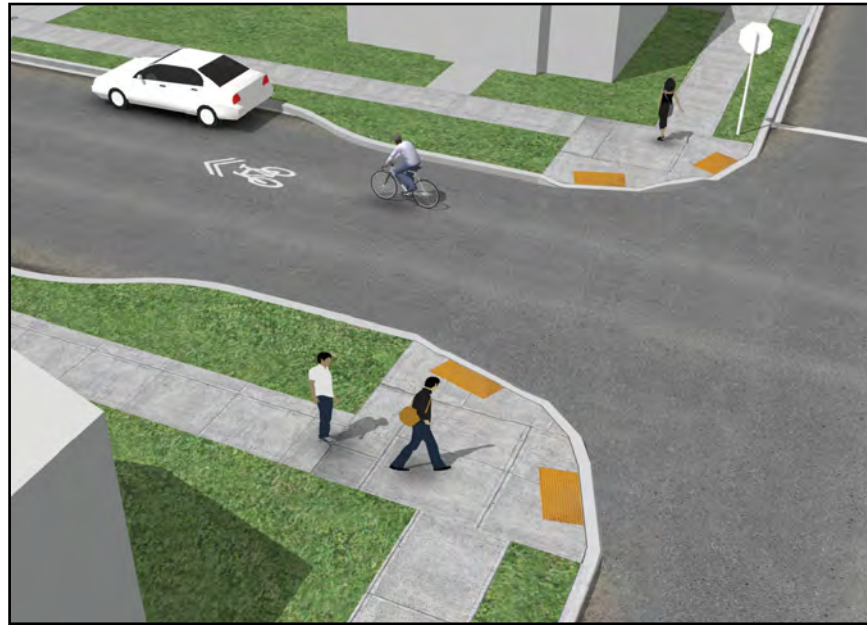
Example of potential Speed Cushion treatment
